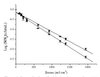
Figure 1. Log reduction of aciduric microorganisms ( $\blacktriangle$ ), molds and yeasts ( $\bullet$ ) after exposure to different doses of UV treatment
